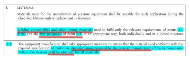
For welding/joining materials, this just needs to a EN10204 type 2.2 certificate, or the equivalent. (A 3.1 or 3.2 certificate is also acceptable). A type 2.2 certificate is a "Document in which the <u>manufacturer</u> declares that the products supplied are in compliance with the requirements of the order and in which he supplies test results based on non-specific inspection."
